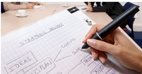
Papershow allows a digital pen to simultaneously display handwritten notes on your computer.
